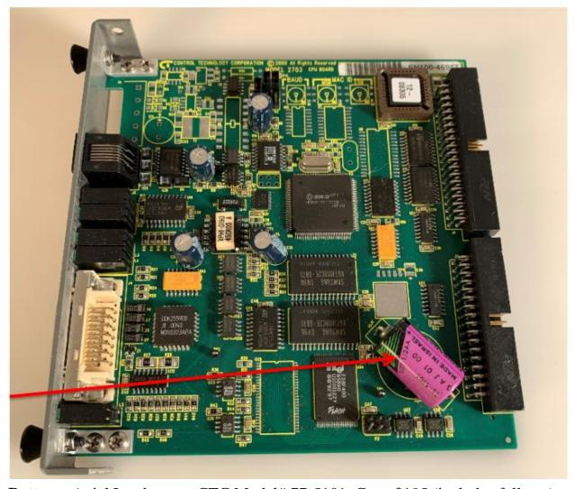
**Battery:** Axial Lead type – CTC Model# 77-5101 Cost: \$195 (includes full test) **Not Field Replaceable – Requires hand soldering ability - Request RMA**
