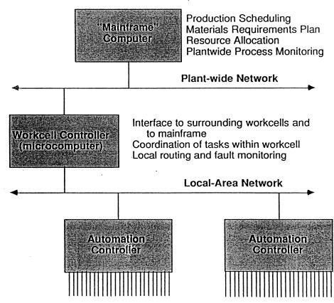
Control over individual actuators on machine tools, automated transfer stations, inspection stations, assembly stations, etc.
