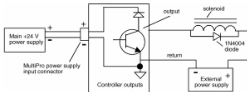
**WARNING:** Each output has a protection diode with its cathode connected to the + 24 VDC power supply at the input connector. This diode prevents damage to the output when connected to an inductive load. If a separate power supply is used for the external devices, as shown above, a current path exists between the two supplies through the devices being controlled. Under normal operation this practice is okay. However some power supplies
