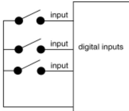
The controller senses when any of the inputs have been pulled down to return by a switch closure, and a Monitor instruction or any other programmed instruction referring to a general-purpose input can use this information.
