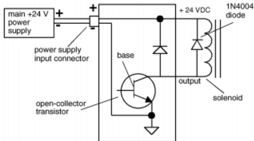
When the output is turned on, current is allowed to flow through the transistor, just as though a switch contact had been closed. The controlled device turns on in response to the flow of current.
