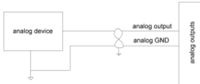
**NOTE:** All shields are located on the controller side and run to ground.
