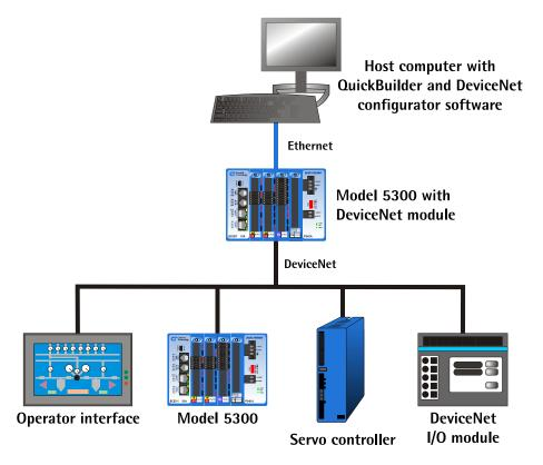
M3-60A: DeviceNet and dual serial port module
