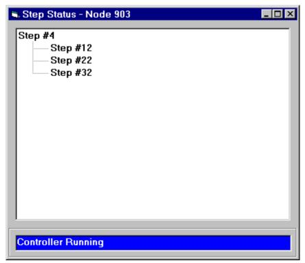
**Controller Status Messages:** The Controller Status Message box indicates the current controller status and displays user prompts.
