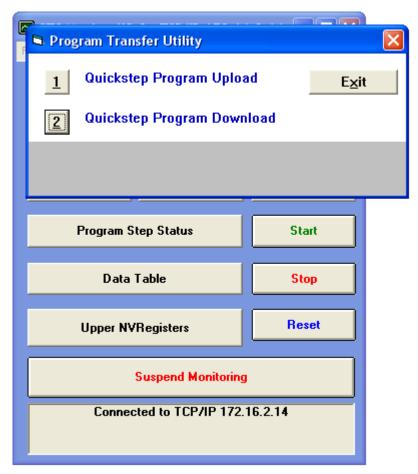
3. To upload the program from your controller to the computer, select the 1 button for **Quickstep Program Upload:**
