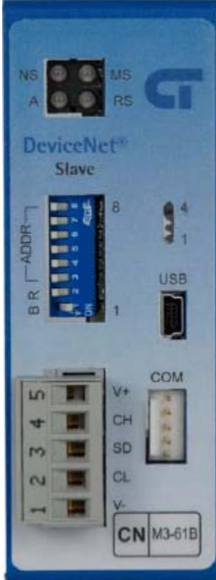
LED – NS, Network Status, green - online, flashing green - no connection, red – link failure.
