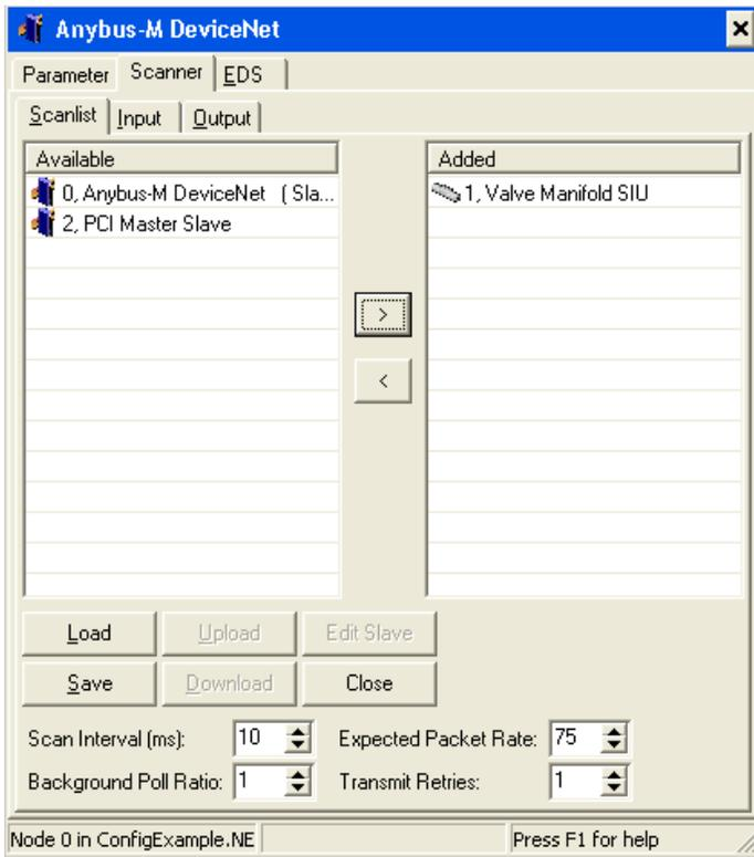
We will now begin to map the I/O of the SMC device. Highlight the device and select the Input tab.
