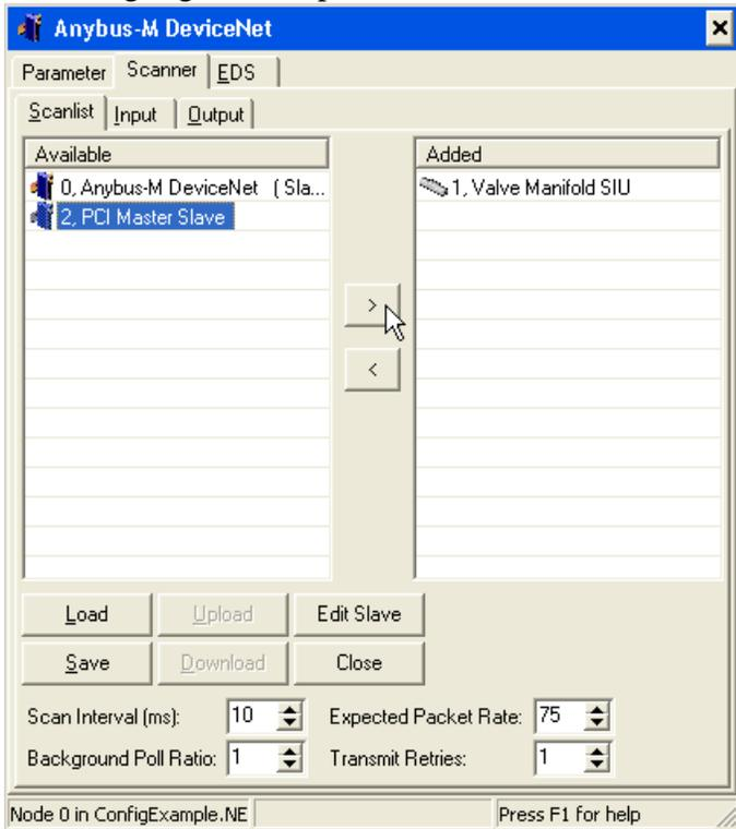
Prior to being added the proposed access methods, bytes received (input) and transmitted (output) are defined. The EDS file defines this as 32 bytes for each or 256 bits of data. In reality you must reference the configuration of the Denso to determine the proper setting or errors will occur. The popup screen below is from page 51 of the *Denso Robot with RC7M Controller \*-G Series Options Manual*, Step 6:
