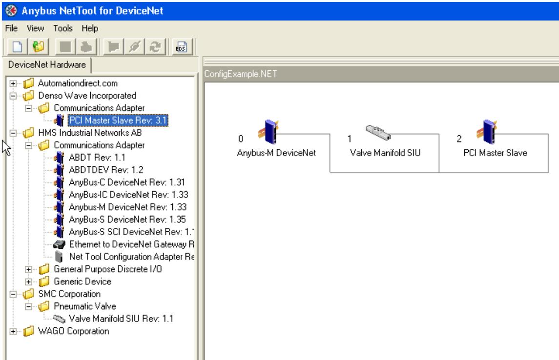
Double click the Anybus-M DeviceNet node in order to get into the scan list configuration screens. If not in Idle mode, use the pull down box, setting it to Idle and then click the Download box, which sets programming mode (only if online):
