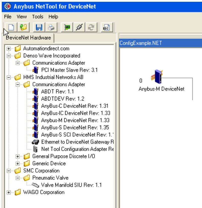
Next drag the SMC Corporation Valve Manifold to the right window. The next sequential MACID is being used as the default (1), but you may set as needed:
