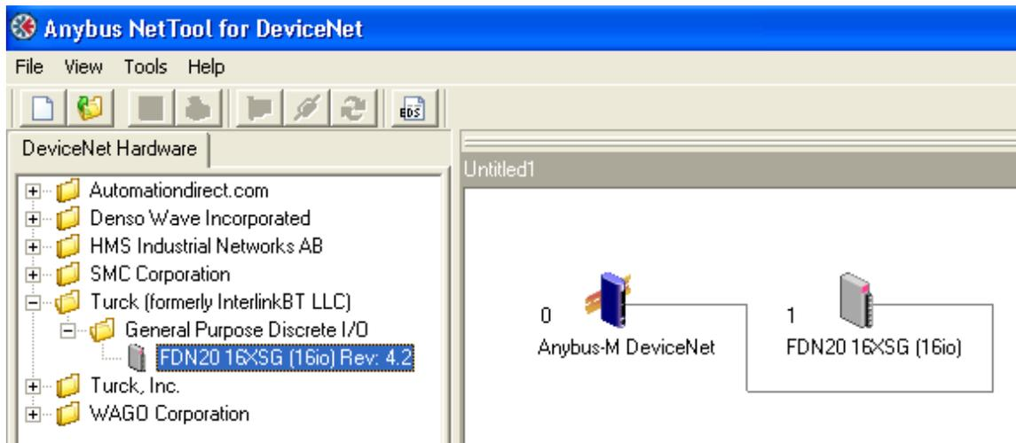
Double click the Anybus-M icon to begin configuration, selecting the 'Scanlist' tab and then move the FDN20 to the active scan list (Added column):
