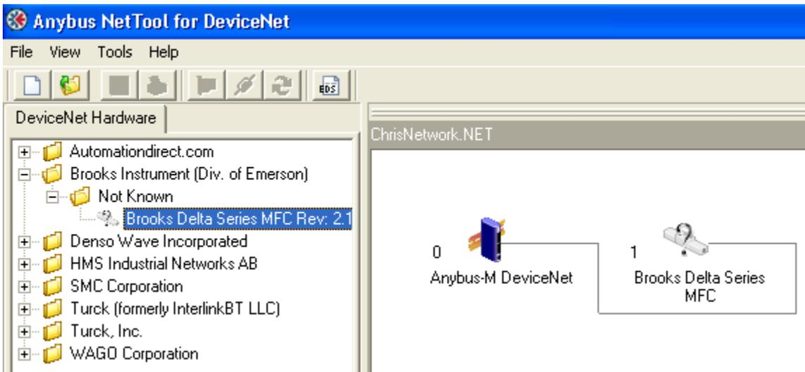
Double click the Anybus-M icon to begin configuration, selecting the 'Scanlist' tab and then move Brooks to the active scan list (Added column):
