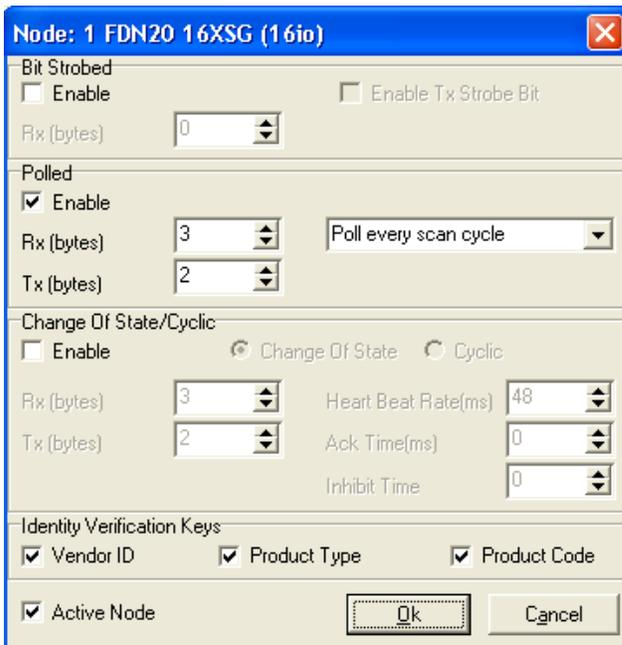
Click OK after any changes and the scan list will appear as below; select the Input tab to begin mapping the produced data (received):
