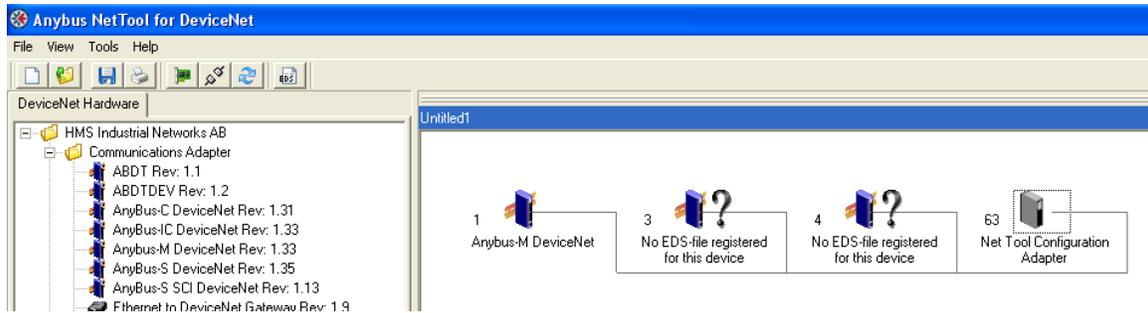
The EDS file can be installed by accessing the Tools menu and selecting Install EDS-file:
