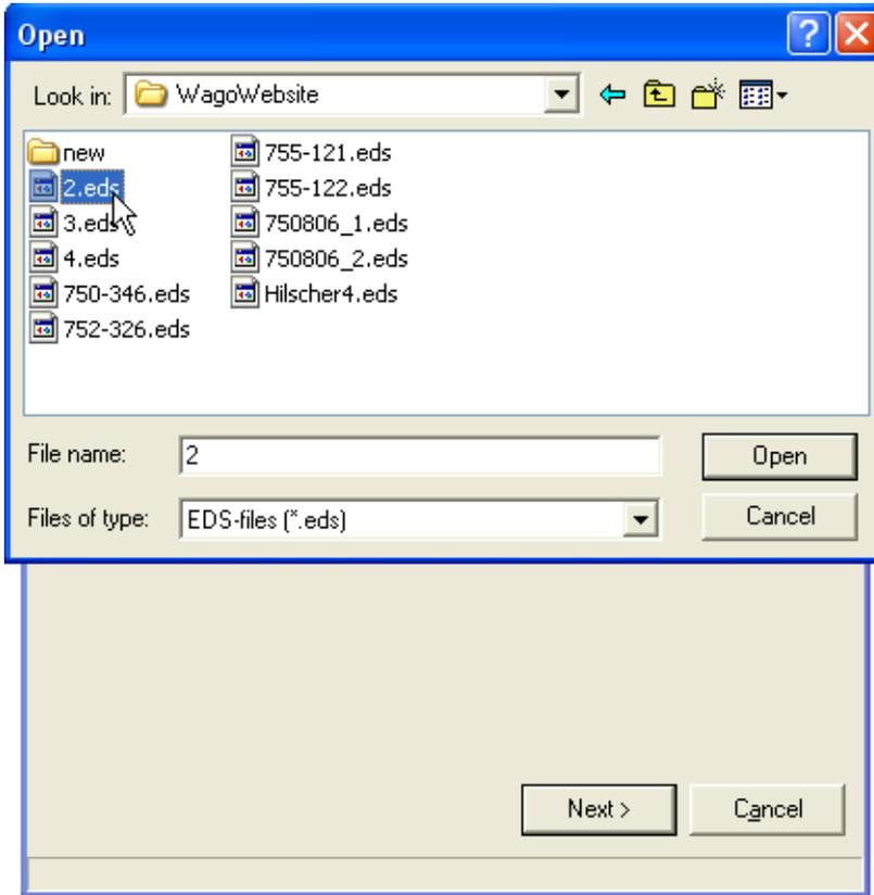
If the EDS file installs successfully the following will appear; a poorly formatted file will give errors:
