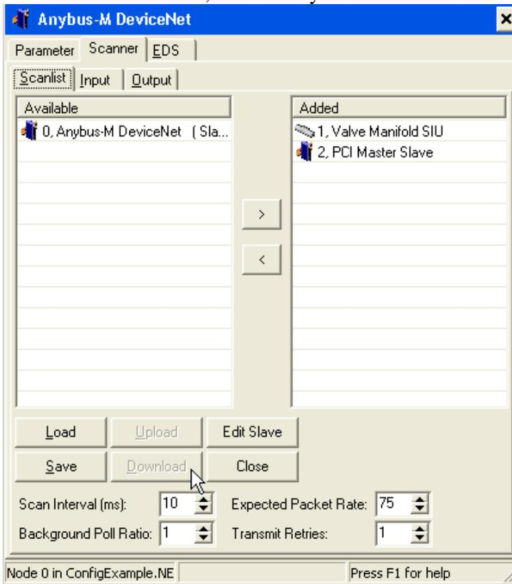
After full configuration it is necessary to cycle power on the Model 5300 controller to ensure that the DeviceNet I/O and local I/O install correctly. The Model 5300 will not operate until all scanned devices that were defined are properly seen as online, as it is assumed that their appearance is required for proper application program execution. You will know things are running properly when all 3 LED's are green and none are red. A flashing red indicator means there is a network setup error.
