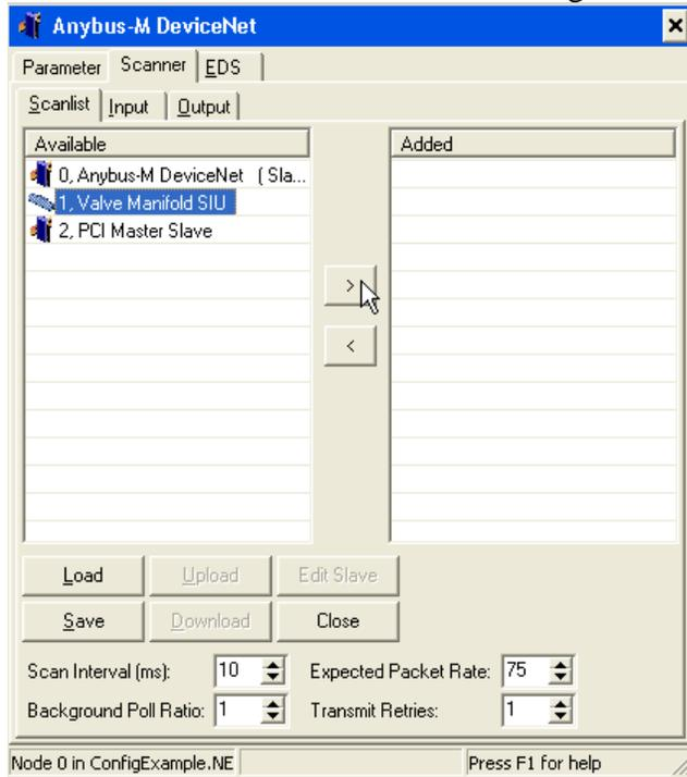
Upon adding, the dialog below will appear requesting the scan information to be entered. All three types are supported by the Master and each block of data returned will be mapped as unique I/O. For the purpose of this example we are assuming Polled only. The dialog below shows that the SMC device returns 6 bytes (48 bits of produced input data) and accepts 4 bytes (32 bits of consumed output data):
