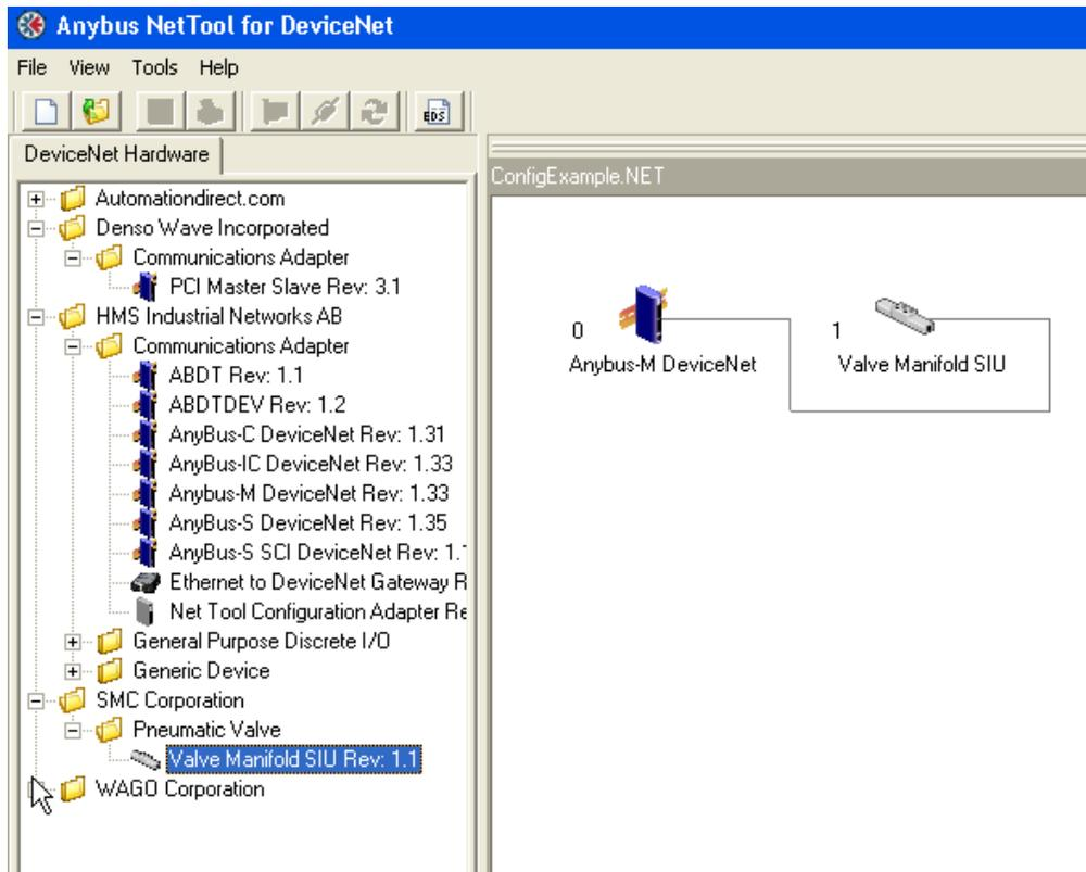
Next drag the Denso PCI Master Slave Device to the network window. The next sequential MACID is being used as the default (2), but you may set as needed:
