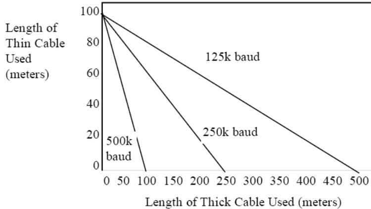
$$L_{\text{thick}} + 5 \times L_{\text{thin}} = 500 \quad \text{at 125Kbaud}$$
