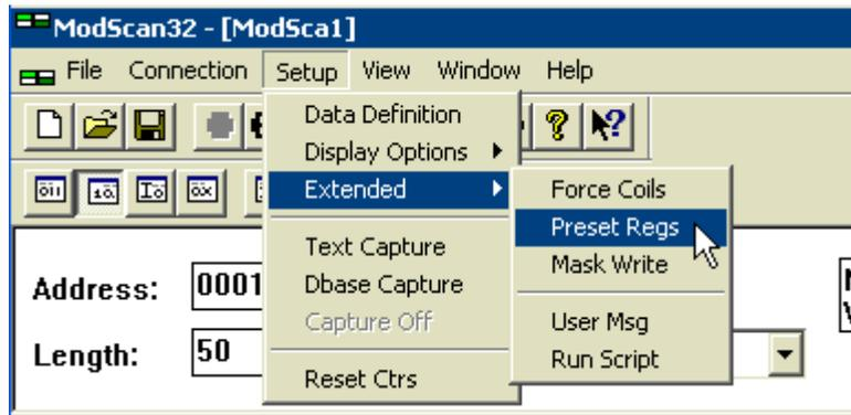
Figure 7.6: Write Multiple register (Preset Regs) selection
