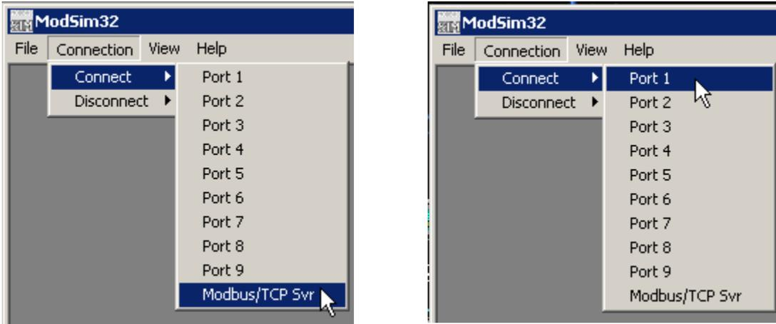
If Serial, select RTU or ASCII and set the baud rate, stop bits, and parity appropriately. Default for the Model 5300 is 19.2K baud, 8 data bits, 1 stop bit, no parity. However, this is not the default for ModSim and must be changed as shown below:
