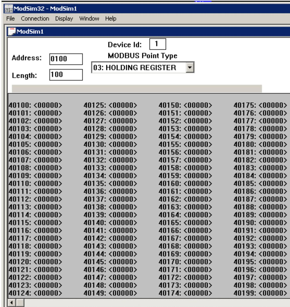
In order to access this device, the controller must have its Device ID set to 1 (the default) and the Starting Address set to 100. If not set correctly, an exception status will be
