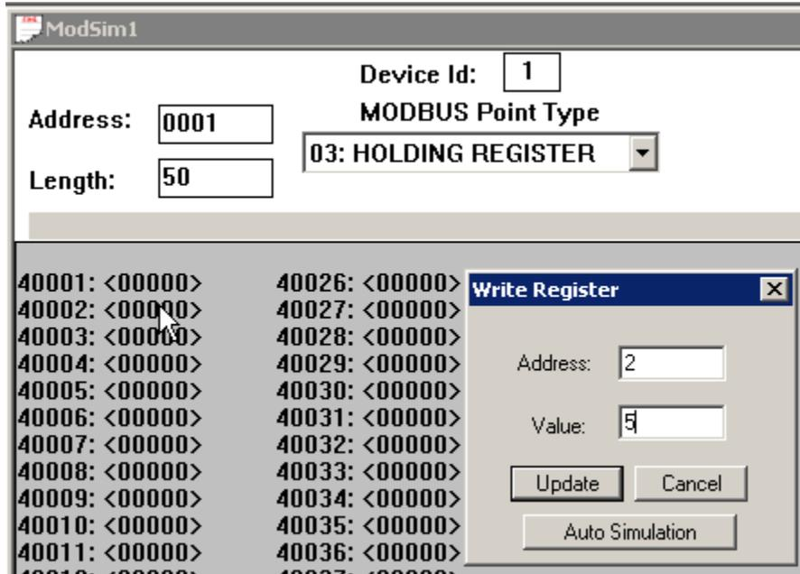
Figure 7.5: Single register write, value 5 to 40002
