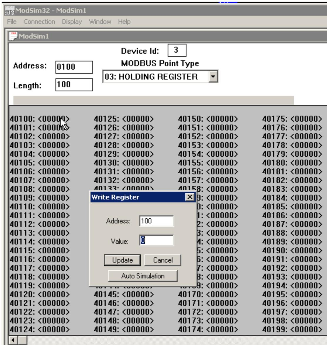
The screen capture above shows the modification of address 100. Additional devices can also be created by once again selecting File->New. This allows for the testing of multiple Modbus Slave devices at the same time:
