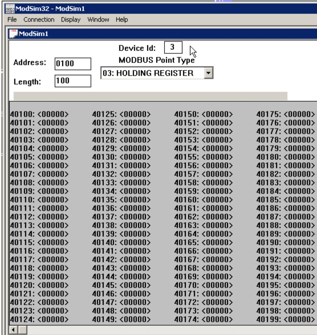
Note that the Address field is set to 100, but the display screen starts at 40100. This is Modbus nomenclature. To modify a device Holding Register contents, simply double click on the address and enter the new value in the dialog that appears:
