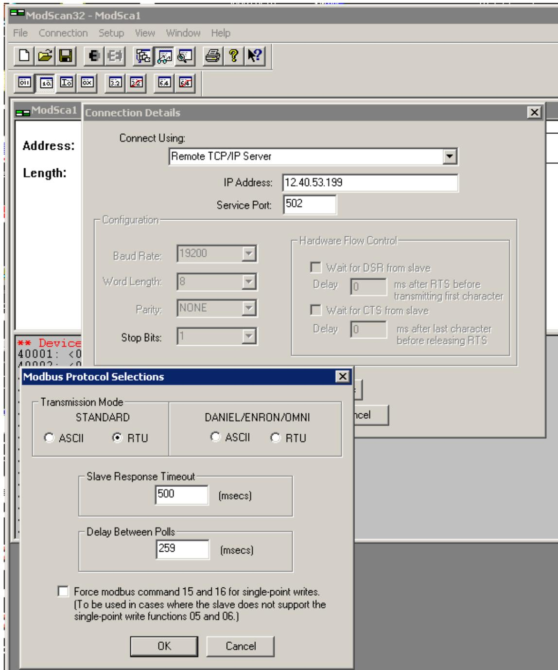
Figure 7.4: ModScan32 Master Scanning Program TCP Connection Setup
