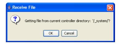
With the proper directory to retrieve the file from verified, select 'OK' and a dialog box of appears allowing you to set where on your computer to place the file being loaded from the controller. Note that the filename you enter must match that on the controller. Press, Save to begin the transfer. Refresh of your screen will stop on large files; this is normal, causing gray or tan areas until complete.
