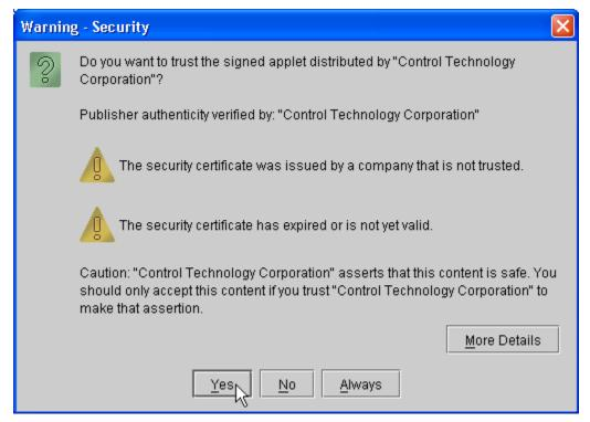
If you fail to authorize WebMON to execute it will appear but nothing will function properly. Authorization of WebMON simply allows it to access local resources, like TCP connections on different IP addresses than the web server, local disk storage, etc.
