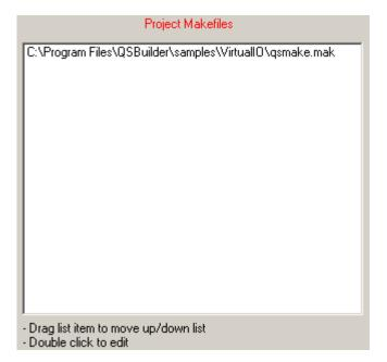
From the Project Builder Screen, select the 'qsmake.mak' file to highlight it, then the 'Build' button in order to Compile and Link the desired files. The output log generated is shown in the next section.
