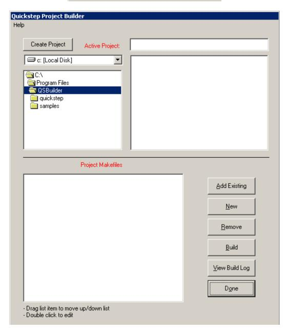
Using the built-in File Manage utility, select the desired directory for creating the project. Then select the 'Create Project' button. A project can be though of as a group of build environments for different Quickstep Programs. In many cases you may only have a single project, although if the program is shared among users, each may have a project file with their own name.
