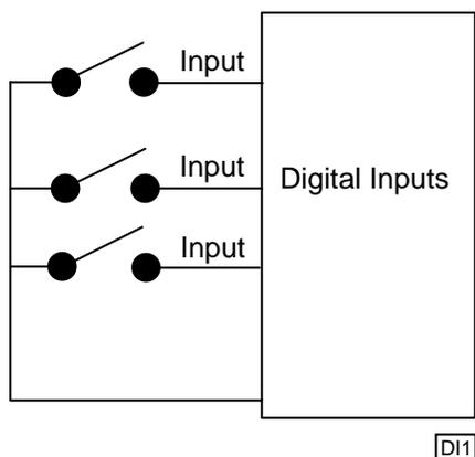
The MultiPro senses when an input is pulled down to **Return** by a switch closure. A `MONITOR` instruction or any other programmed instruction referring to a general purpose input can use this information.
