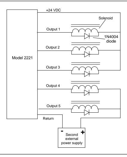
**IMPORTANT!** Do not use an external power supply with an output voltage greater than the output voltage rating of the outputs.
