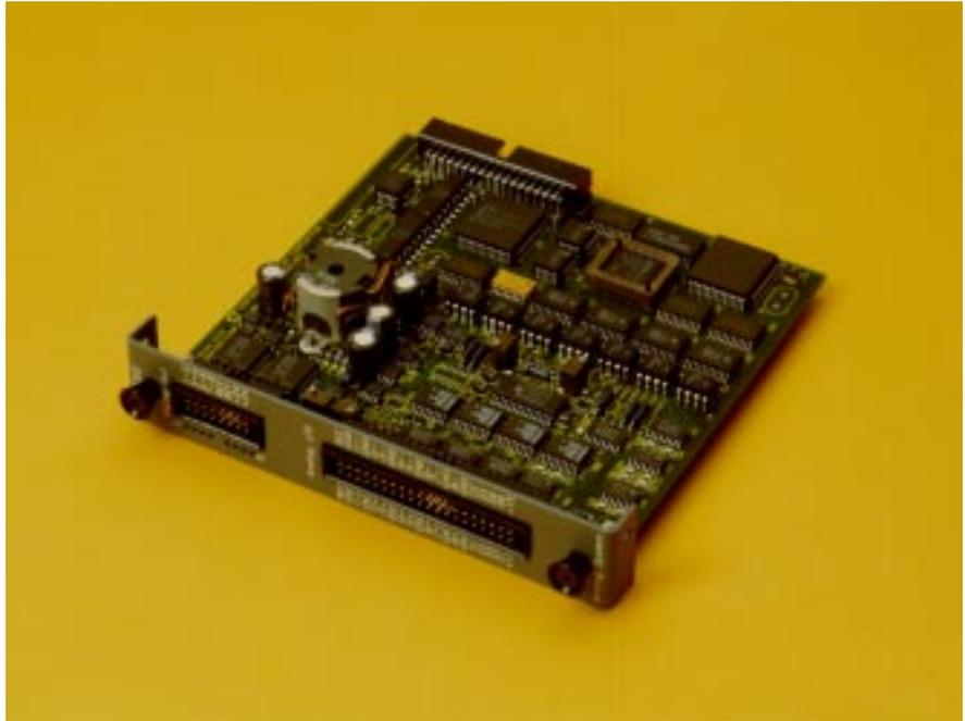
The 2220 analog subsystem provides 8 differential analog inputs, 8 analog outputs and 8 digital outputs in a single module. The bipolar ( $\pm 10$  Volt) analog inputs offer 15 bit resolution, and may be individually programmed to digitally filter the incoming signal, providing increased stability. From 2 to 256 analog samples may be continuously averaged at an update rate of 2.083 milliseconds.
