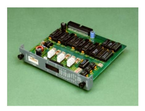
The model 2208 High-Speed Counter Module accepts a quadrature signal from a range of industry-standard optical encoders, tracking the resultant count at rates up to 1 million "edges" (counts) per second. Useful for position checking and for velocity determination, the model 2208 may be configured for either single-ended or differential-output encoders.
